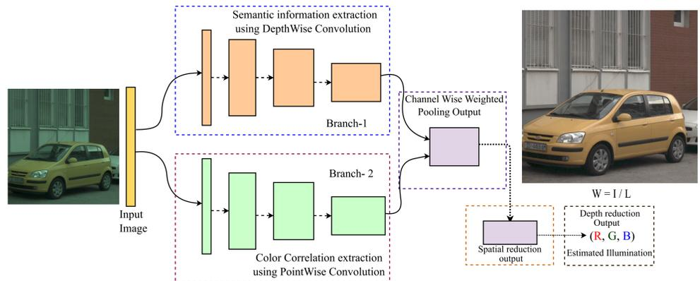
Dual branch architecture for color constancy depicting respective output tensors of each layer.
