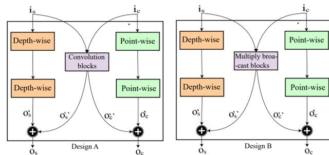
The two design variants of micro-block architecture for soft parameter sharing over baseline method. Non-linearization and pooling layers are not shown for a better depiction.
